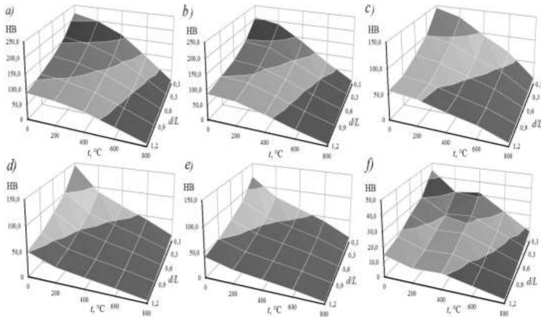
**Figure 1 a, b, c, d, e, f** – Patterns of changes in the hardness of HB of various materials used in friction units, on temperature  $t$  and the relative value  $d/L$  ( $d$ ,  $L$  are the diameter and friction path of the contact patch): a - steel 30KhGSA; b - cast iron ChNMKh; c – FPM brand FMK-845; d – FMK-11; e - FPM brand MVK-50A; f - retinax FK-16L
