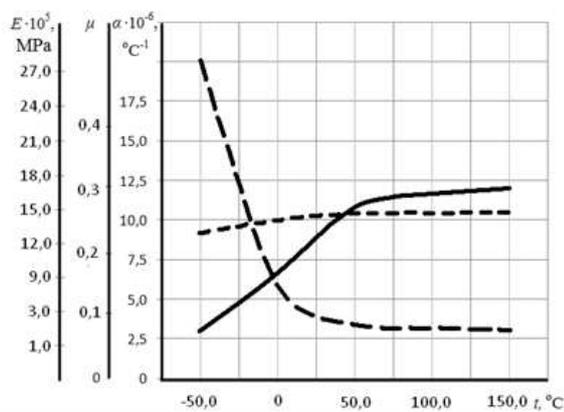
**Figure 2** – Experimental dependences of the modulus of elasticity  $E$  (—), Poisson's ratio  $\mu$  (---) and linear expansion coefficient  $\alpha$  (—) steel 30HGSA on temperature  $t$ .
