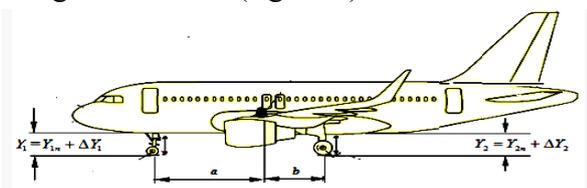
**Figure 1** – Vertical displacement of fuselage of the aircraft
