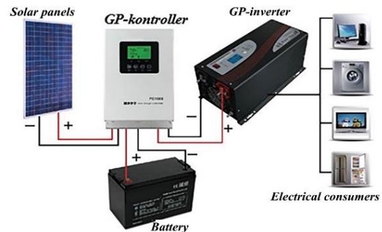
Figure 9 – Power circuit of APSSP Inverter: for single phase-network: MUST EP3000 (12-14/220 V, 1-6 kVt); GW15K-DT (26 kVt and higher) GP-controller-solar panel controllers: (MPPT-controller): PC1600F; series 45/60/80A (MPPT)
