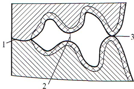
**Figure 7** – Scheme of contact of microprotrusions of metal-polymer friction pairs: 1, 3 – contact zone with destroyed and undamaged film (metal contact zone); 2 – no contact zone
