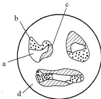
**Figure 2** – Model of contact surfaces of microprotrusions of friction pairs: a – “metal-metal”; b – “polymer-metal”; c – “polymer-polymer”; d – non-contacting spots of microprotrusions
