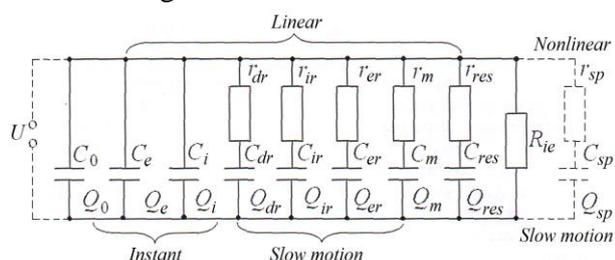
**Figure 8** – Equivalent electrical circuit of a polymer pad
