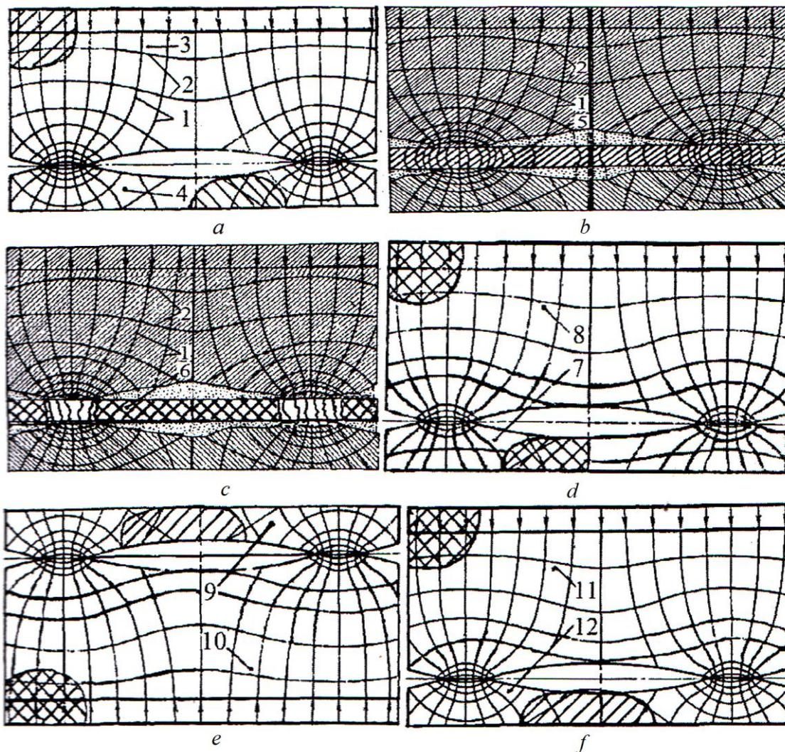
**Figure 4** – Thermal current lines (7) and isotherms (2) during frictional interaction of contacts of friction pairs: a – “metal (3) - metal (4)”; b – “metal (3) - metal film (5) - metal (4)”; c – “metal (3) - polymer film (6) - metal (4)”; d – “polymer (7) - polymer (5)”; e – “metal (9) - polymer (10)”; f – “polymer (11) - metal (12)”
