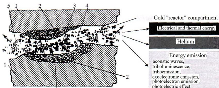
**Figure 1** – Magma-plasma model: 1 - initial structure; 2 - molten structure; 3 - plasma; 4 - triboemission electrons; 5 - atoms, photons, phonons, ions, excited molecules, fast electrons
