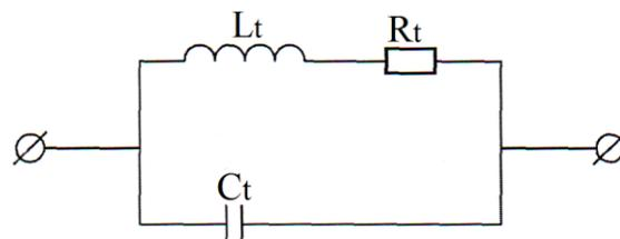
**Figure 5** – Equivalent circuit of electrical contact of microprotrusions of friction pairs
