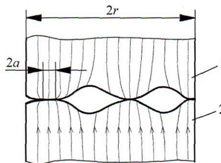
**Figure 3** – Lines of electric current contraction in discrete contacts of microprotrusions of the friction pair “polymer (1) – metal (2)”
